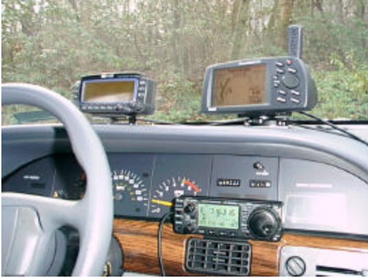
Photo 5. Chas Richard, W4HFZ's mobile APRS Satellite capability (including HF. very short APRS style communications via any 9600 Baud PACSAT with digipeat enabled (UO-22)).
