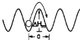
Fig. 1. Representation of carrier motion by way of hopping between potential wells. \Delta H and a correspond to well depth or trapped site binding energy and well separation, respectively [4,5].
