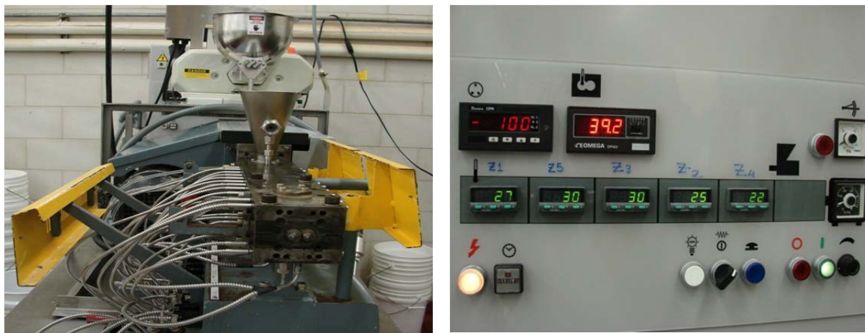
Fig.A1 Extruder and a close view of the five temperature zones.
