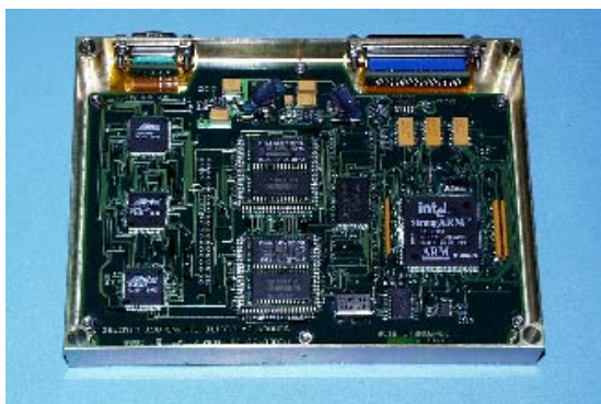
Fig. 8. SNAP-1 On-Board Computer
