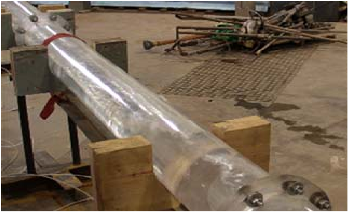
Figure 3: 7-inch model showing pipe supports
