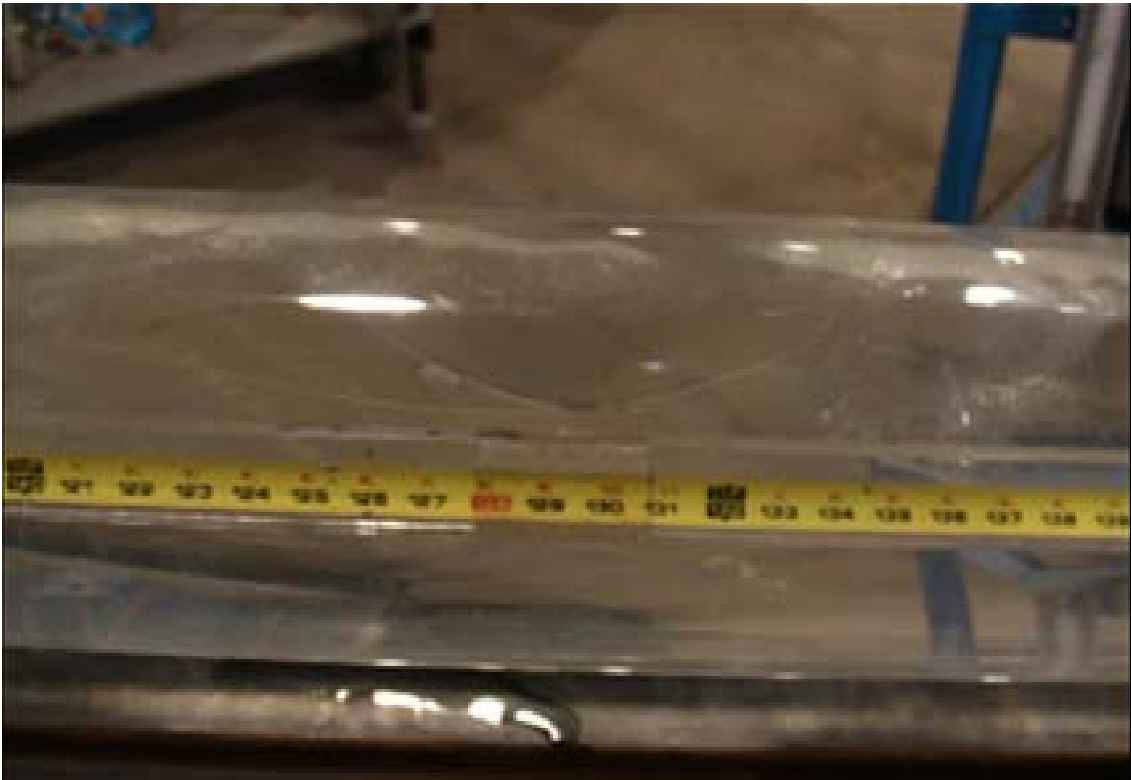
Figure 5: Large scale attached to 7-inch model
