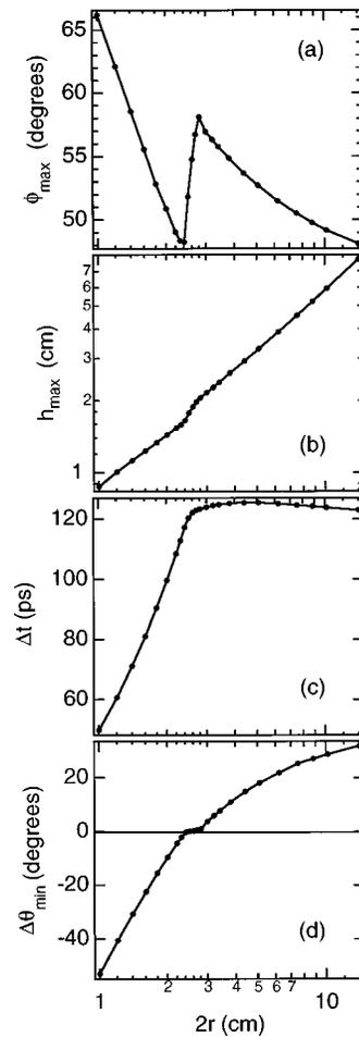
FIG. 2. Results of calculations optimizing the mirror angle  $\phi$  and beam height  $h$  for maximum delay time  $\Delta t$  as a function of the mirror separation  $2r$ . (a) Optimum mirror angle  $\phi_{\max}$ . (b) Optimum beam height  $h_{\max}$ . (c) Resultant delay time  $\Delta t$  for corresponding  $\phi_{\max}$  and  $h_{\max}$ . (d) Difference in minimum rotation angle conditions  $\Delta \theta_{\min} = \theta_{\min,2} - \theta_{\min,1}$  (see the text for details).
