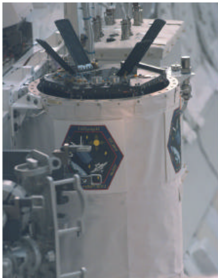
Figure 3: MightySat I in Hitchhiker Can
