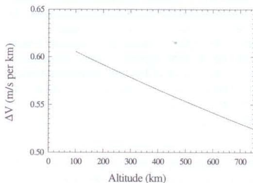
Figure 1.  $\Delta v$  required for orbit raising
