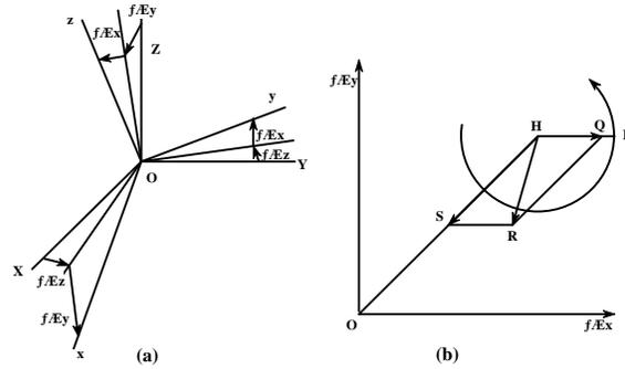
Fig.5 Principle of Pointing. (a) Target Attitude C XYZ and body-fixed coordinate O-xyz.  $\alpha, \beta, \gamma$  are small Euler angles. (b) shows a free nutation of satellite in  $x-y$  plane.
