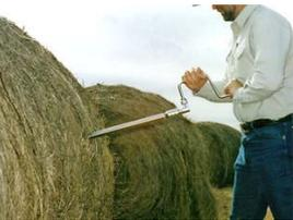
Figure 15. Core sampling of a round bale
