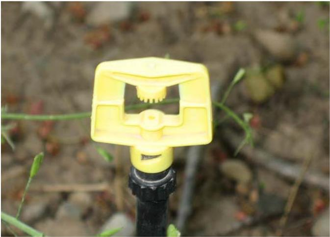
If runoff is occurring, the rate of application should be reduced to match the rate of soil water intake. Sprinklers are convenient for small acreage situations, but do require a continuous supply of water during operation. Small amounts of water (0.5 to 2 acre-inches per acre) can be applied more uniformly with sprinklers than with surface methods. Thus, sprinklers are suitable for coarser textured soils and shallow rooted crops.
