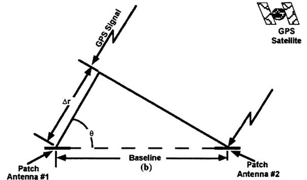
Figure 6. GPS Interferometry
