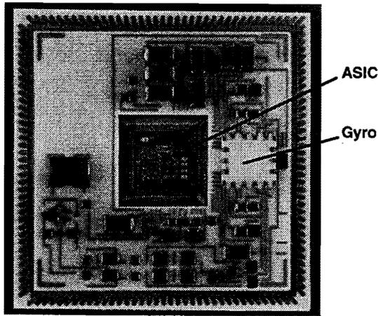
Figure 4. 2.5-cm by 2.5-cm Gyro and ASIC Package
