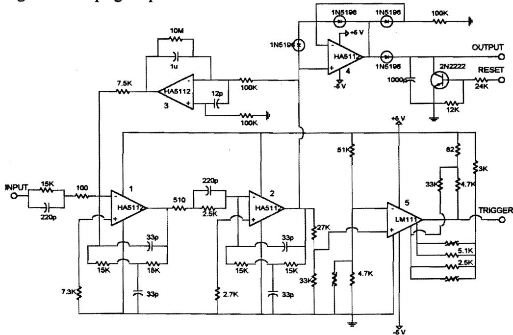
Op-amp #4 is part of the sample and hold circuit for the amplifier. The additional circuitry (op-amp and diodes) has the effect of eliminating the diode drop that occurs in a conventional S/H. The typical diode drop is undesirable in this case, particularly when the pulse output from the amplifier has a magnitude significantly less than 5 V.
