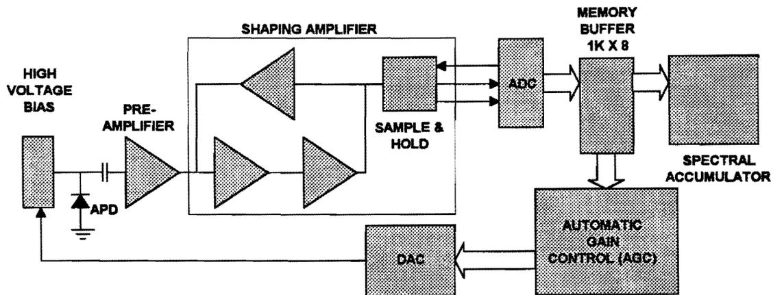
4.4 are necessary for the continuous adjustment of the high voltage bias to the APD. The processing of a calibration event is similar to a normal events up until the memory buffer. At this point the digitized calibration pulse is read by the Automatic Gain Control (AGC) which will adjust the gain of the APD.
