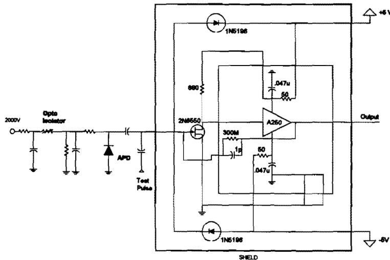
It utilizes an external FET, for impedance matching to the APD, and will be cooled by radiation along with the APD to -40 C when CATSAT is in flight. This cooling is achieved by placing the detector and preamplifier in the SXR module on the top of CATSAT's spaceframe, this also maximizes the distance between the noise sensitive components and the satellites operational controllers.
