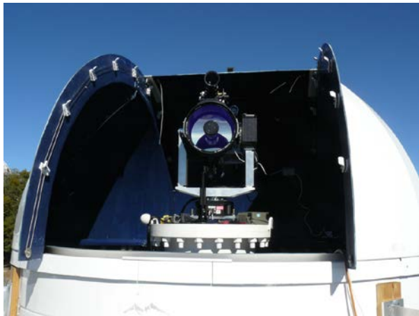
Figure 5. Photograph of our 30-cm diameter Meade receive telescope in our MOCAM optical ground station.
