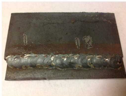
Figure 2. Weld test coupon.
