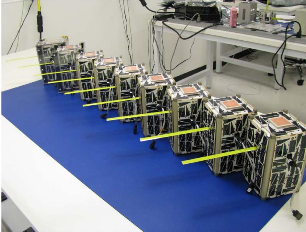
**Figure 2: EDSN Spacecraft Ready for Flight (eight flight units, one flight spare)**
