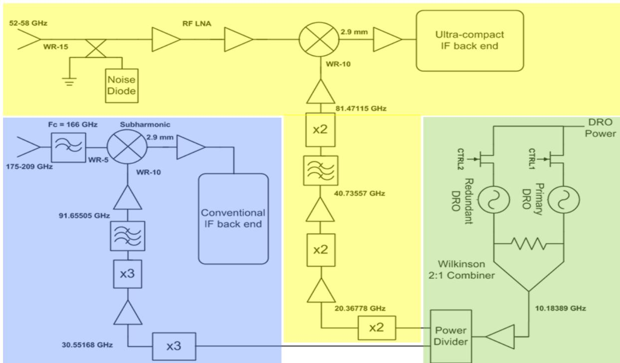
**Figure 1:** The MiRaTA tri-band, 10-channel microwave atmospheric sounder provides all-weather temperature, humidity, and cloud ice measurements for weather forecasting and climate studies. The V-band (yellow) and G-band (blue) receiver systems are completely independent, with a redundant dielectric resonator oscillator (green) common to both.
