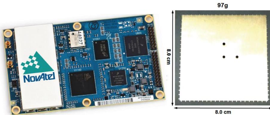
**Figure 7:** The NovAtel OEM628 GPS receiver is shown on the left, and one of the dual-band GPS patch antenna/LNAs is shown on the right. The GPSRO element of CTAGS (nominally zenith facing) consumes < 2W and the precision orbit determination element of CTAGS (nominally ram facing) consumes ~1.3W.
