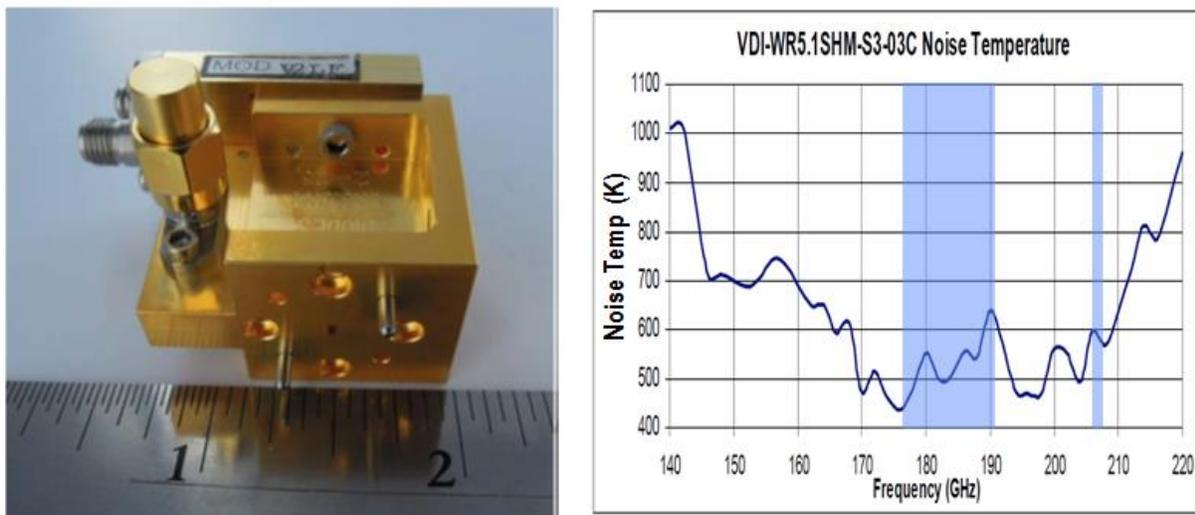
**Figure 5:** The Virginia Diodes, Inc. (VDI) wideband mixer front end will provide double-sideband measurements in three channels near the water vapor absorption band ( $183.31 \pm 1$ ,  $\pm 3$ , and  $\pm 7$  GHz), and a single-sideband measurement of a 206.4 to 208.4 GHz cloud ice band.
