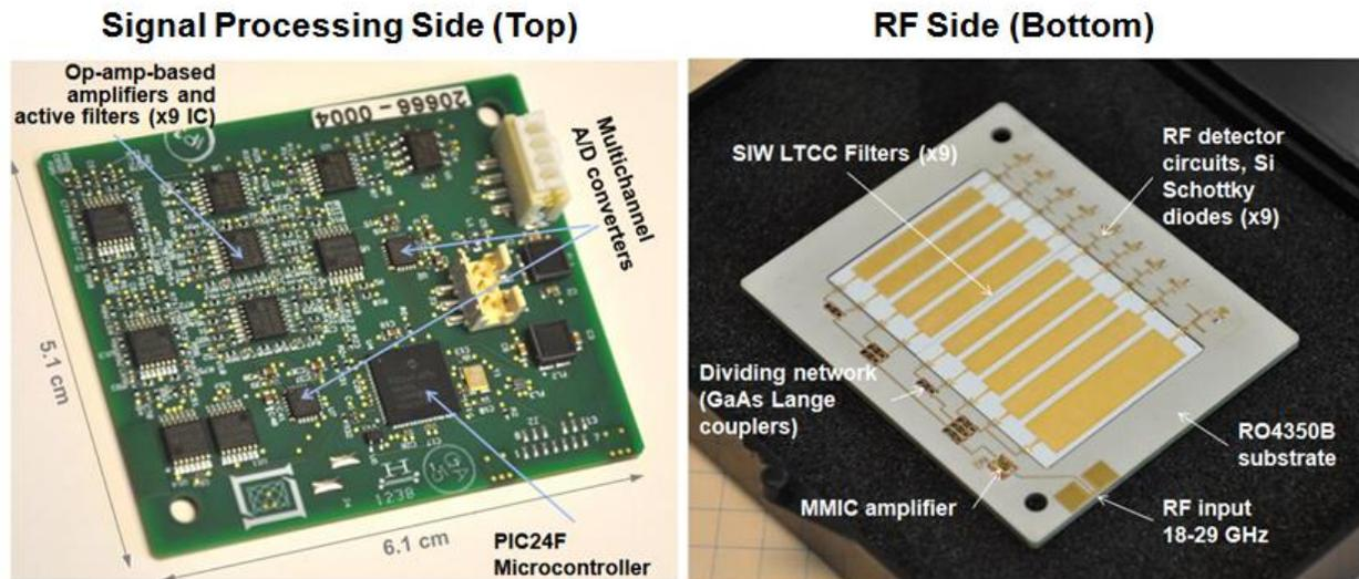
Figure 4: The ultra-compact spectrometer to be used in the MiRaTA V-band radiometer. The top side of the board contains analog and digital signal processing electronics and interfaces to the control and data handling (C&DH) radiometer module. The bottom side of the board contains the microwave components needed for power division, amplification, filtering, and detection. A lightweight, RF-tight enclosure has been fabricated using metal-coated, metal-infused ULTEM.
