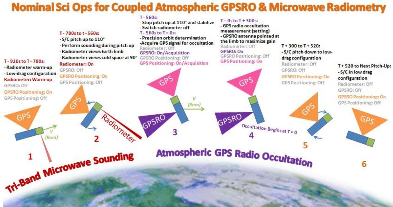
**Figure 3:** The MiRaTA primary mission validation concept of operations (ConOps) is shown above. A slow pitch maneuver ( $\sim 0.5^\circ/\text{sec}$ ) is used to scan the radiometer fields of view through the Earth's limb and subsequently direct the CTAGS field of view through the same atmosphere to catch a setting occultation. The entire maneuver takes about 20 minutes and is performed once per orbit over a 60-day validation period (approximately 1000 total scans).
