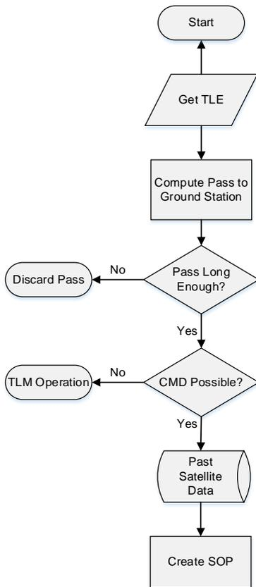
**Figure 4: Satellite Operations Procedures (SOP) Generation Flow**
