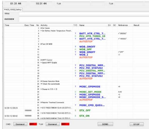
**Figure 5: Example of Satellite Operations (TT&C) Terminal.**
