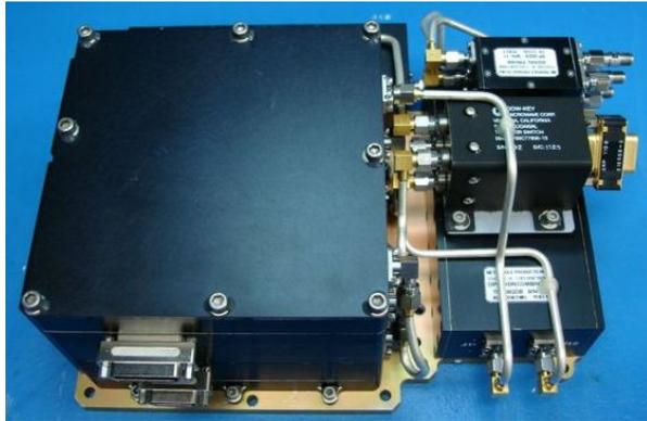
**Figure 1: Space Micro's Integrated  $\mu$ STDN Transponder. The core transponder is on the left. The diplexer, RF switch and test couplers are on the right.**
