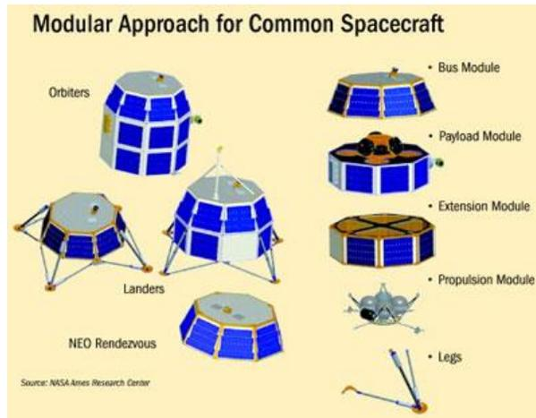
**Figure 1 – Modular Approach for Common Spacecraft<sup>2</sup>**
