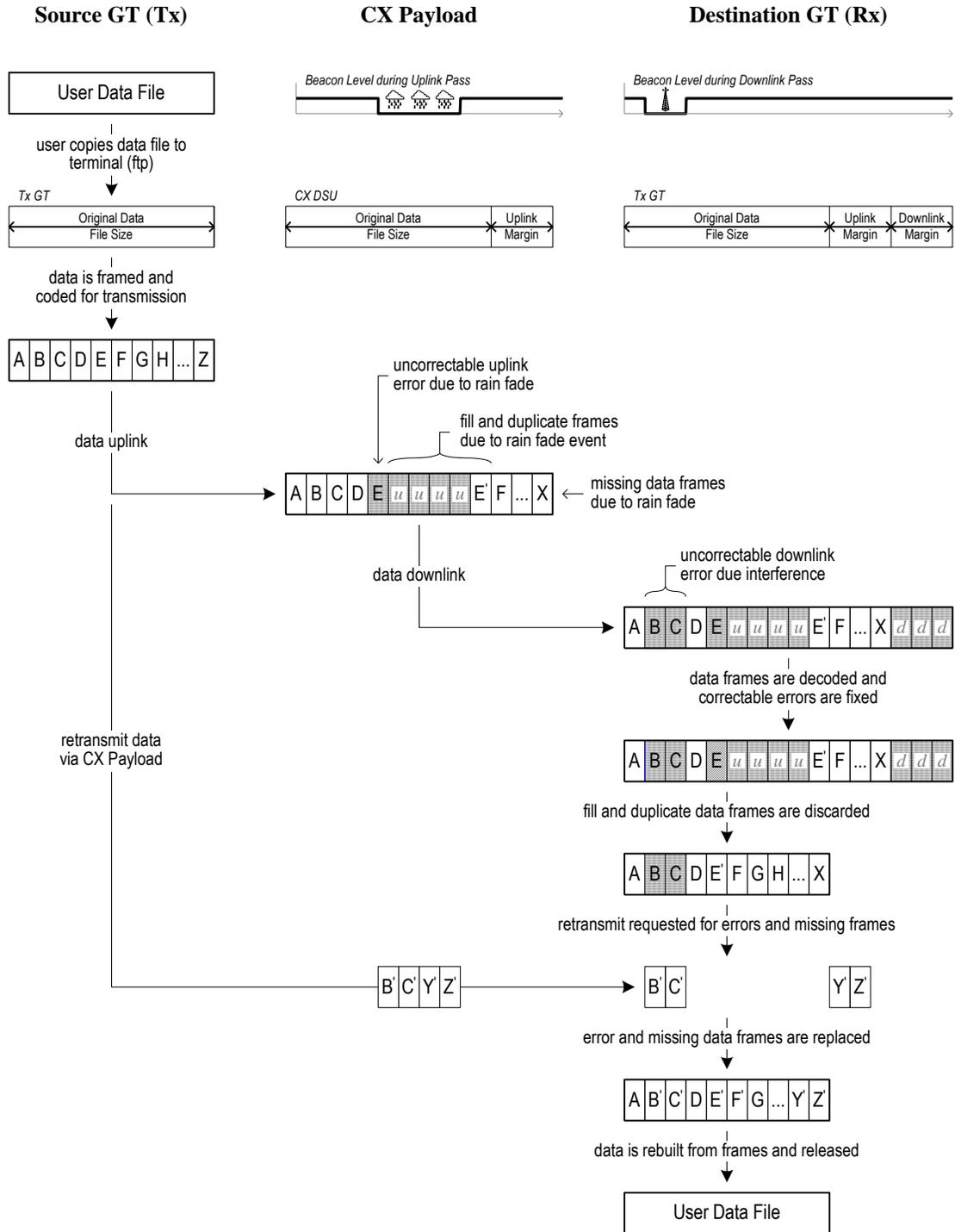
**Figure 7: CX Re-Transmission Case**
