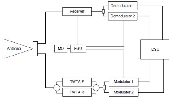
**Figure 1: Block Diagram of CX Payload**
