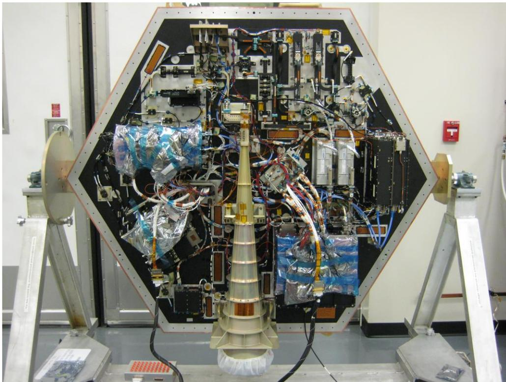
**Figure 2: CX Payload installed on Payload Panel**
