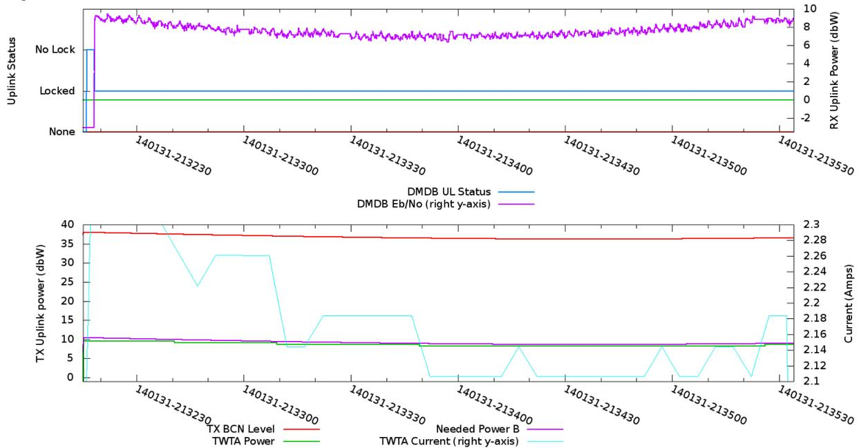
Figure 8: CX Signal and Power Telemetry During Uplink from GT
