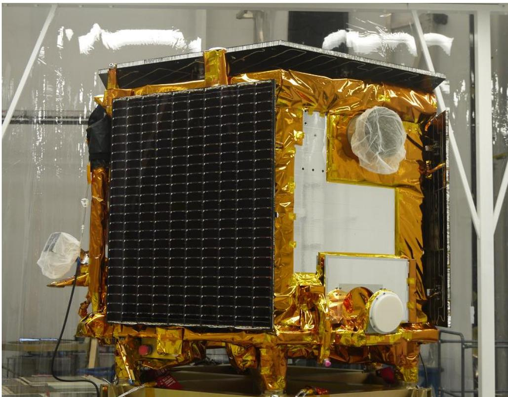
**Figure 3: CX Payload installed on CASSIOPE Spacecraft**
