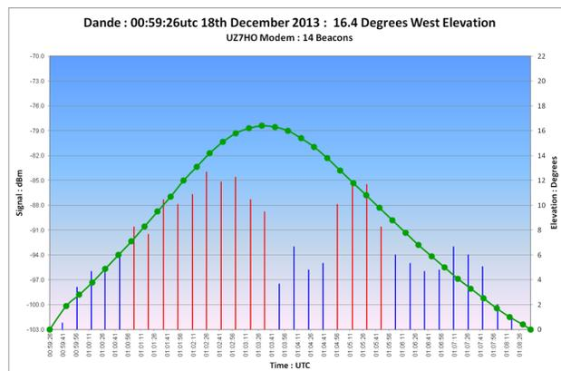
**Figure 5. Received Signal Strength, Showing the Mid-Pass Link Drop**
