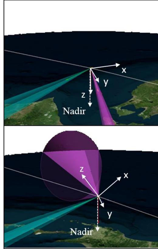
**Figure 4 Ambiguity in attitude determination using EHS readings. The scenario in the second subfigure yield the same sensor readings as in the first subfigure while the satellite's z-axis is no longer in alignment with the nadir vector.**
