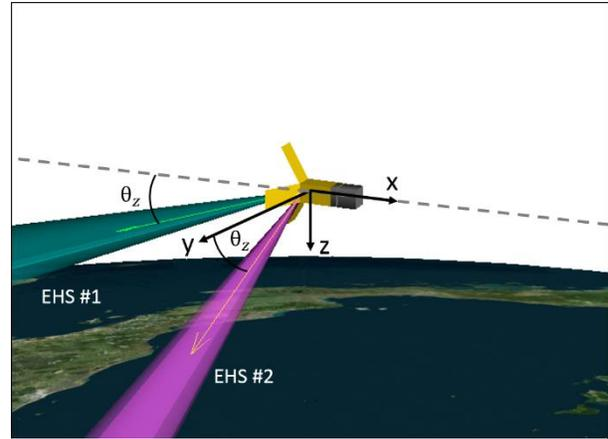
**Figure 1 EHS mounting configuration in the satellite's body frame**
