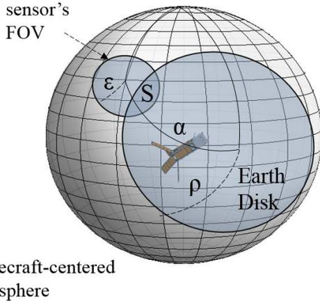
**Figure 2 Projections of the sensor's FOV and the Earth on the spacecraft-centered unit sphere<sup>1</sup>**
