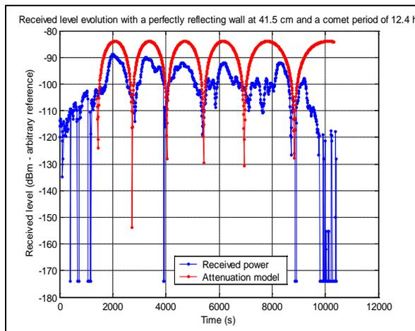
**Figure 13: Comparison of attenuation model with RSSI**
