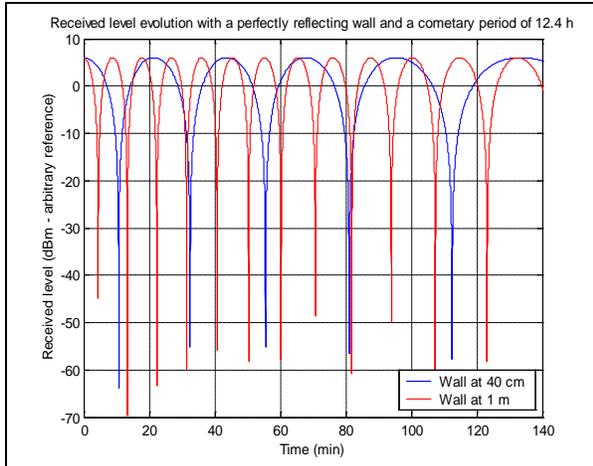
**Figure 12: Variable attenuation model for reflecting surface at 1 m and 0.4 m**
