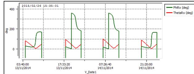
**Figure 10: Lander antenna azimuth and elevation angles simulation during FSS**
