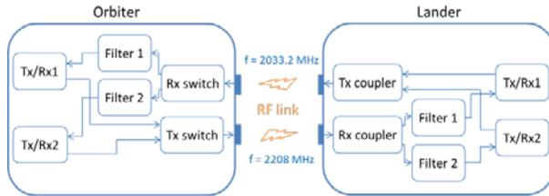
**Figure 1: Rosetta-Philae bidirectionnal RF link**
