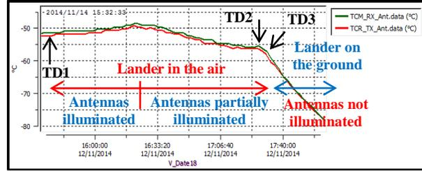
**Figure 8: Lander antennas temperature from first touchdown up to end of RF visibility window**
