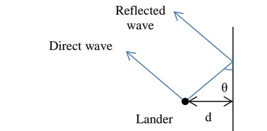
**Figure 11: Wave reflection model**
