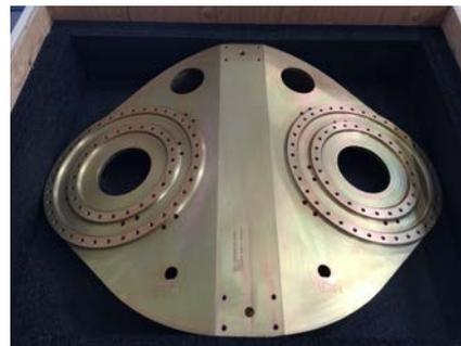
**Figure 11: Flight dual payload adapter**
