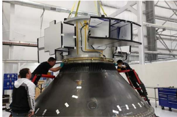
**Figure 9: SHERPA fit check with volumetric models**
