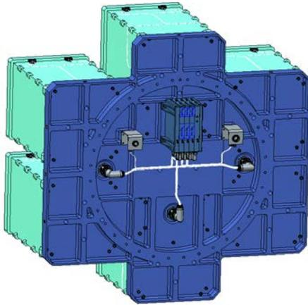
**Figure 7: QuadPack Plate integrated with dispensers and electronics**
