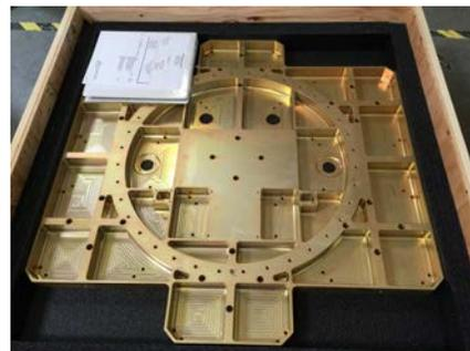
**Figure 10: Flight QuadPack Plate**
