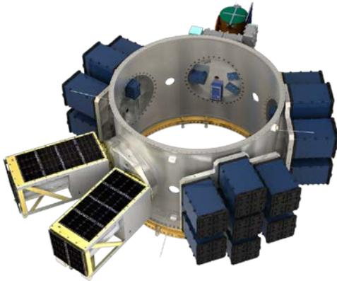
**Figure 1: 2015 SHERPA Flight Configuration**
