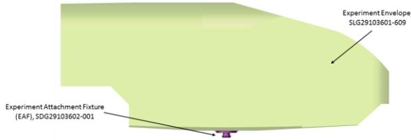
**Figure 9: Cyclops Experiment Envelope**
