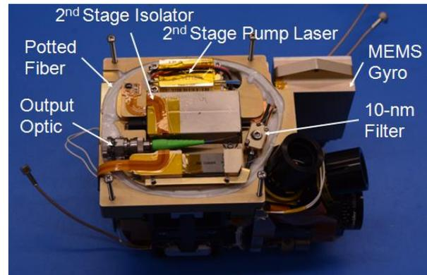
**Figure 7. Photograph of the laser transmitter.**
