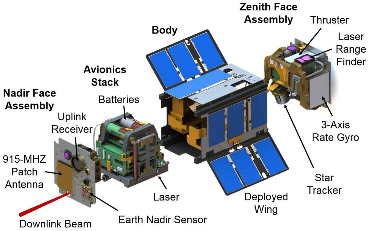
Figure 4. Exploded schematic view of the AeroCube-OCSD CubeSat.
