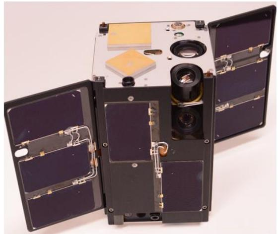
Figure 3. Photograph of the Pathfinder spacecraft with solar wings deployed; alternate view.
