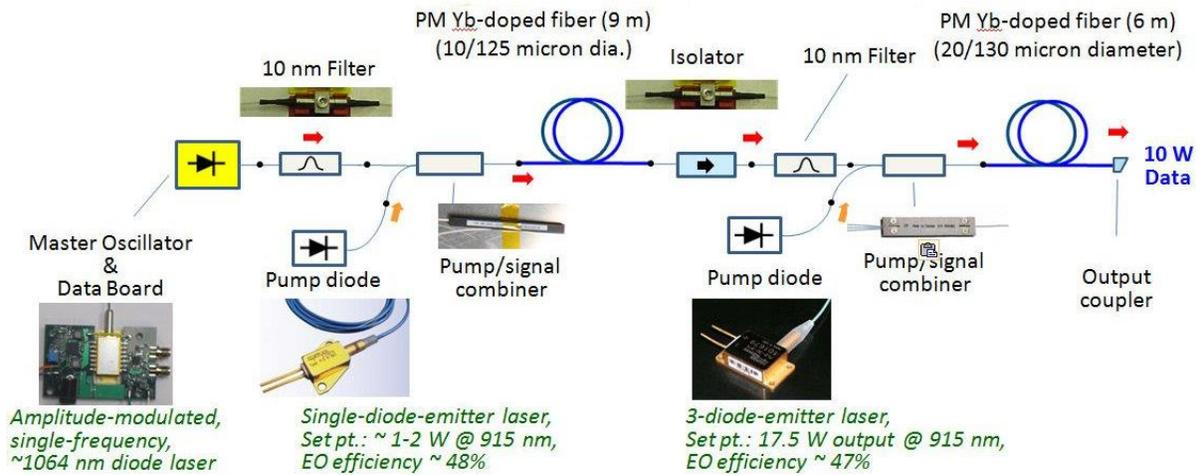
**Figure 5. Schematic diagram of the laser transmitter.**
