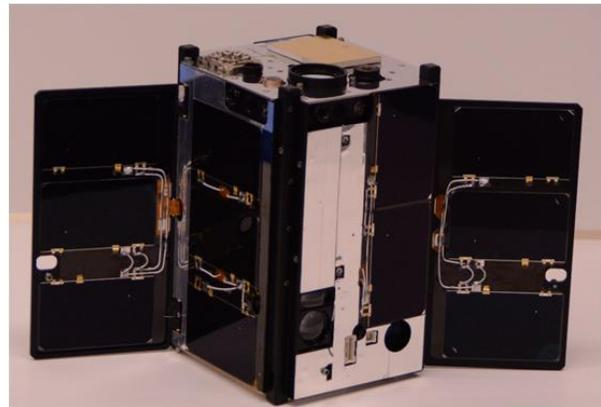
**Figure 1. Photograph of the Pathfinder spacecraft with solar wings deployed.**
