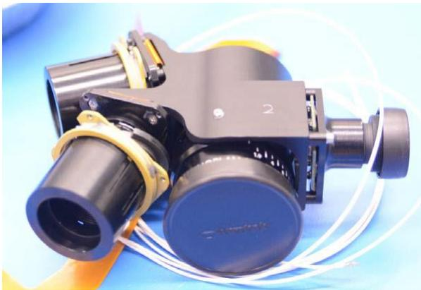
**Figure 10. Photograph of the assembled star tracker (left), Earth imaging camera (bottom middle), and side-looking camera (right side) module.**
