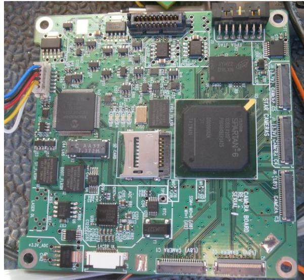
**Figure 8. Photograph of our star tracker/ image processing board.**
