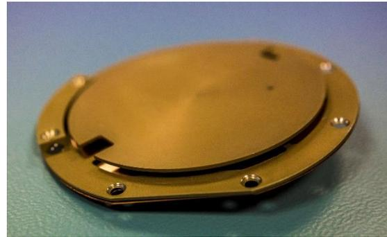
**Figure 10 - S-Band patch antenna**
