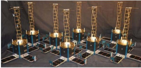
**Figure 3: Prometheus Block 1 Satellites Just Prior to Stowing and Integrating into the Dispensers**
