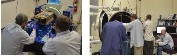
**Figure 11: Block 1 Random Vibration (Left) and Thermal Vacuum (Right) Testing**
