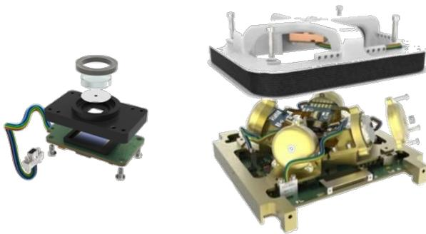
**Figure 7: Sun Vector Sensor (Left) and Block 1 ADCS Module (Right)**
