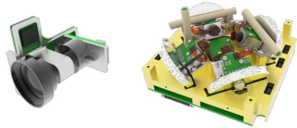
**Figure 8: Star Field Sensor (Left) and Block 2 ADCS Module (Right)**
