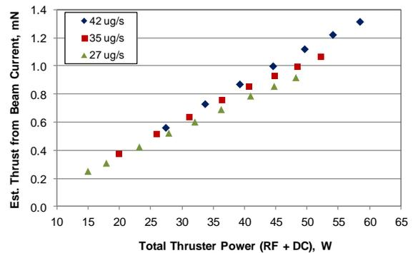
**Figure 6: Iodine BIT-3 Estimated Thrust vs. Total Thruster Power**
