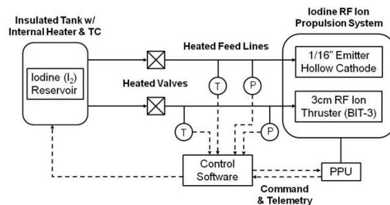
**Figure 4: Iodine BIT-3 System Block Diagram**
