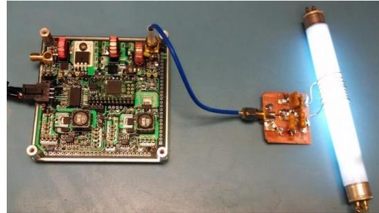
Figure 9: Demonstration of Novel RF Generator/Amplifier Board within the BIT-1 PPU
