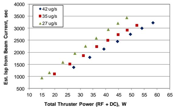
**Figure 7: Iodine BIT-3 Estimated Isp vs. Total Thruster Power**
