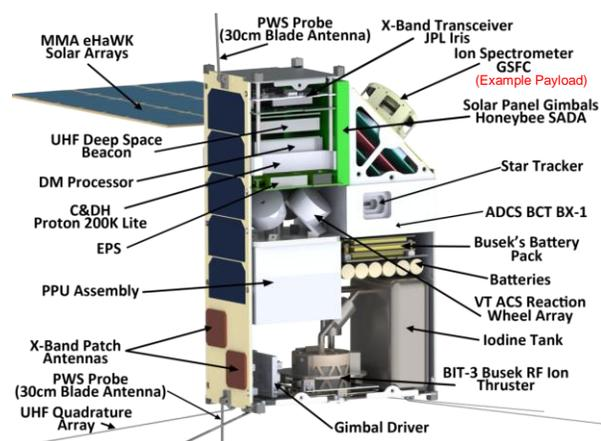
**Figure 2: Up-to-Date Design Layout of the 6U Lunar Cube with Example Science Payload**
