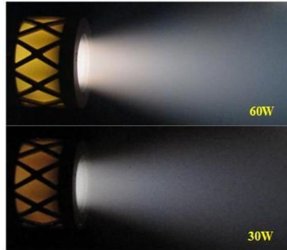
**Figure 5: Iodine BIT-3 Operating at Different Total Thruster Power Levels**
