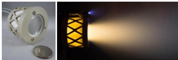
**Figure 1: BIT-3 RF Ion Thruster Firing with Iodine Propellant at 60W Thruster Power**
