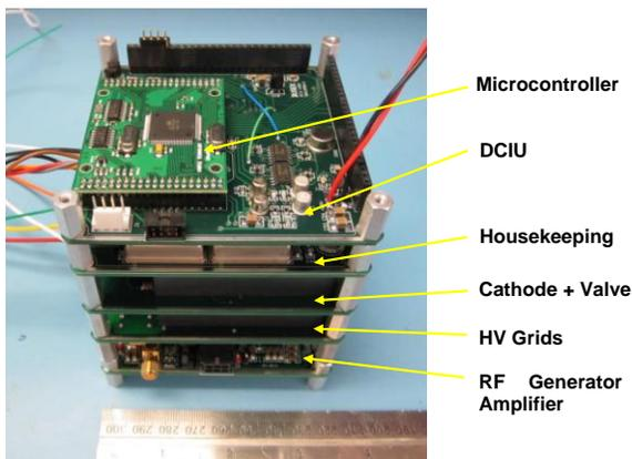
Figure 8: Complete, Breadboard Style BIT-1 PPU
