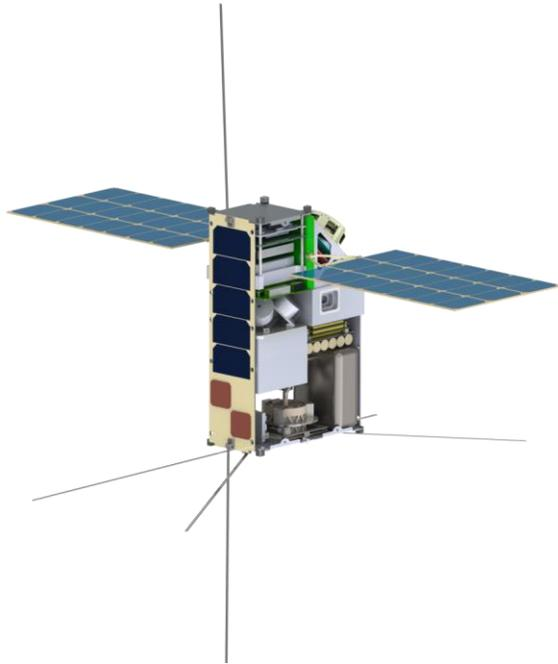
**Figure 3: Complete View of the Baseline Design for the 6U LunarCube Spacecraft**
