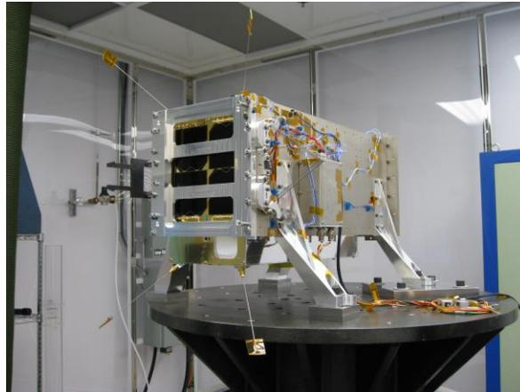
**Figure 1: GHGSat-D in its XPod deployment mechanism, during vibration testing**
