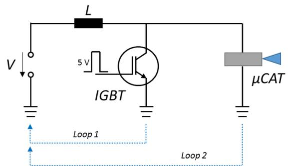
**Figure 2: Thruster circuit diagram**
