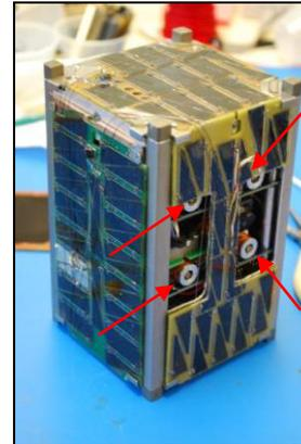
**Figure 4: BRICSat-P 1.5 U CubeSat with four GWU micro cathode arc thrusters (see arrows).**
