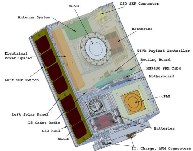
**Figure 4. SORTIE Observatory Configuration**
