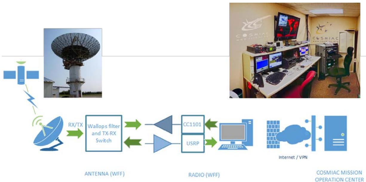
**Figure 5. SORTIE Mission Operations Schematic**
