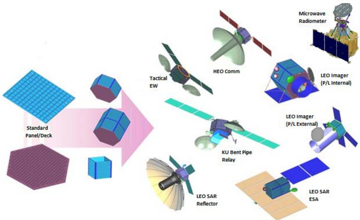
Figure 1: The many configurations of the MSV Architecture
