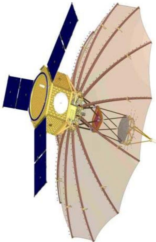
**Figure 2: The ORS-2 bus configuration with the SAR payload**
