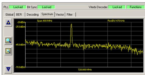
**Figure 3: Spectrum of the received X-band signal from the GOMX-3 satellite**
