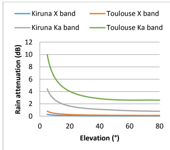
**Figure 4: Rain attenuation for 1% of unavailability in X and Ka bands for Toulouse and Kiruna stations**
