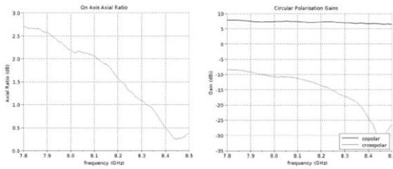
**Figure 2: Syrlinks X-band patch antenna measurement results**
