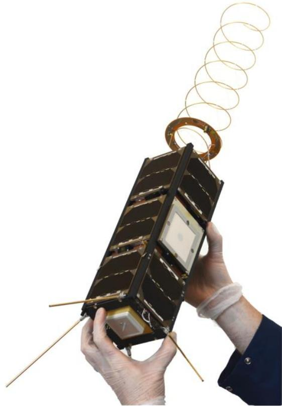
**Figure 1: The GOMX-3 satellite showing Syrlinks X-band patch antenna**
