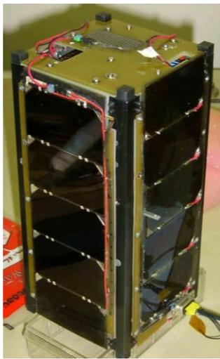
**Figure 1: ION, the University of Illinois' first nanosatellite**
