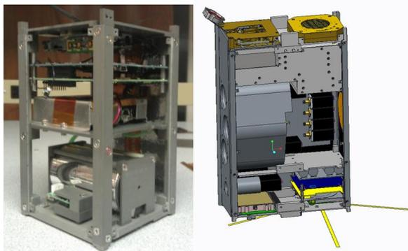
**Figure 4: Partially assembled CubeSail 1.5U satellite (left) and the LAICE 6U satellite (right)**
