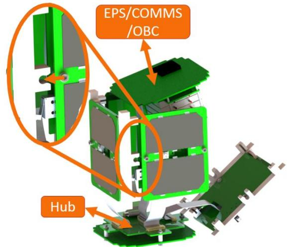
**Figure 11: The two remaining sides are snapped into rails, leaving only one side assembly not attached.**
