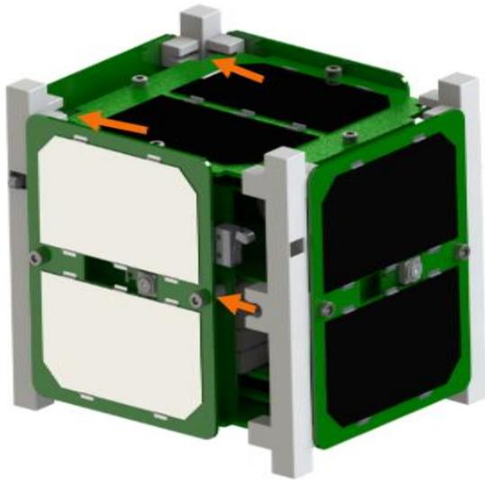
**Figure 13: The Hub and EPS/COMM module are slid into their respective slots in the 3D printed rails.**
