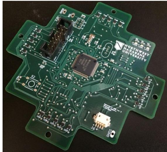
**Figure 5: The Hub board showing the MSP430FR6989 microcontroller, science board interface hardware, and JTAG programming port. The connectors to the other MakerSat electrical boards are located on the reverse side (not shown).**
