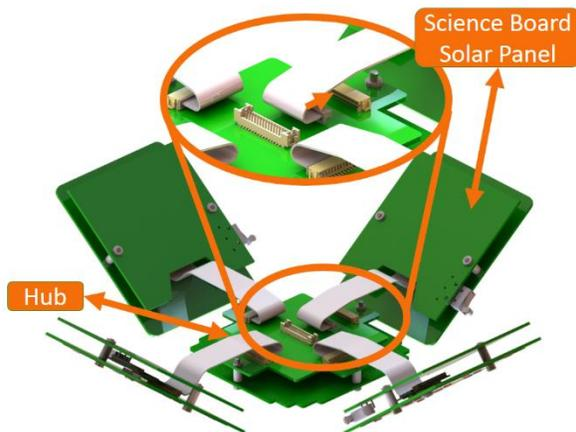
**Figure 8: Four solar cell array/science board assemblies are plugged into the Hub.**
