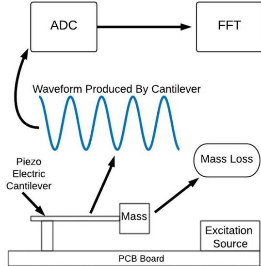
**Figure 6: A diagram of the polymer mass loss experiment. The 3D printed polymer to be tested is attached to the end of a piezoelectric cantilever and excited by a vibration source. The resonant frequency of the voltage output by the cantilever is related to the mass of the 3D printed polymer by (1). By comparing the resonant frequency of the 3D printed polymer to the resonant frequency of a reference mass, the change in mass due to space exposure can be determined.**
