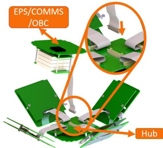
**Figure 9: The EPS/COMMS module is plugged into the Hub.**
