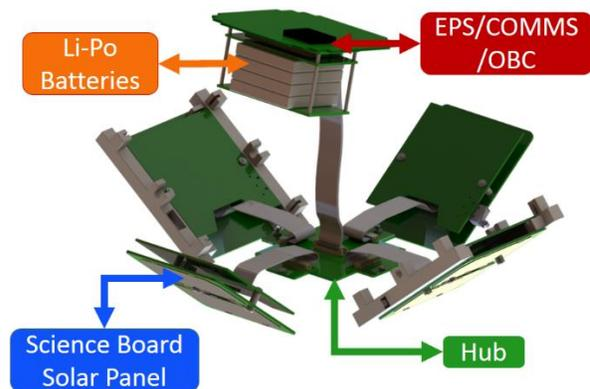
**Figure 2: An exploded view of the MakerSat showing the OBC/EPS/COMMS board, batteries, each solar panel array/science board assembly, and the Hub (bottom solar panel array omitted for clarity).**
