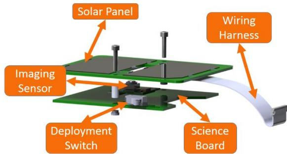
**Figure 3: Four sides of the CubeSat will consist of a science board mounted directly behind the solar panel array. The science board contains an imaging sensor that will protrude between solar cells and a deployment switch mounted between the two PCB's.**
