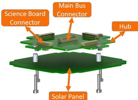
**Figure 4: The Hub is mounted directly to the bottom solar array for ease of assembly.**
