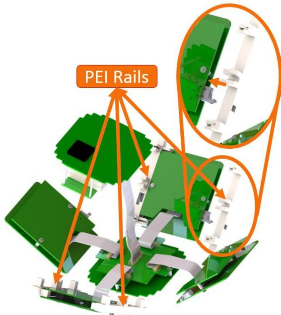
**Figure 10: The 3D printed rails are snapped into place on opposite sides of the CubeSat.**
