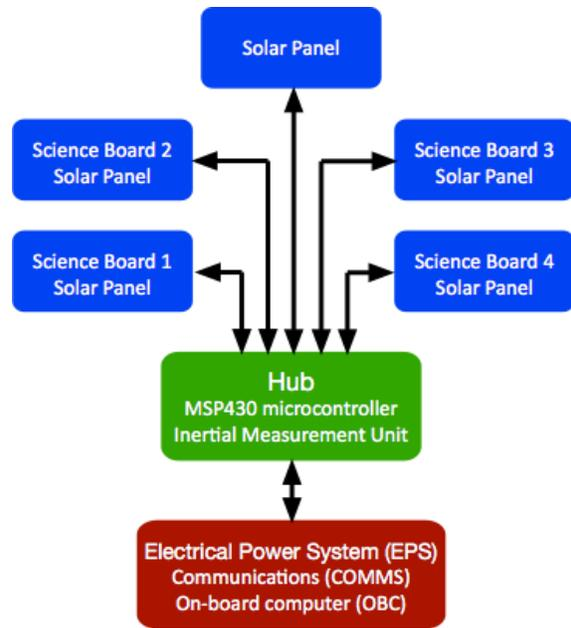
**Figure 1: The MakerSat system block diagram showing the central Hub, electrical subsystems (i.e., the EPS, COMMS, and OBC), and the multiuser science boards and solar panel arrays.**
