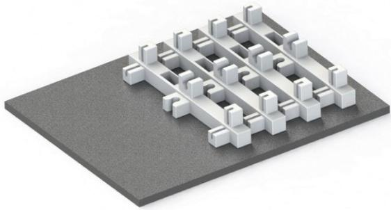
**Figure 7: The MakerSat-1 3D printed PEI rails on the print bed. The rails were designed to be 3D printed without support material.**
