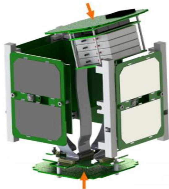
**Figure 12: The Hub and EPS/COMMS are then pushed together towards the center of the CubeSat and lined up with their respective slots in the rails.**
