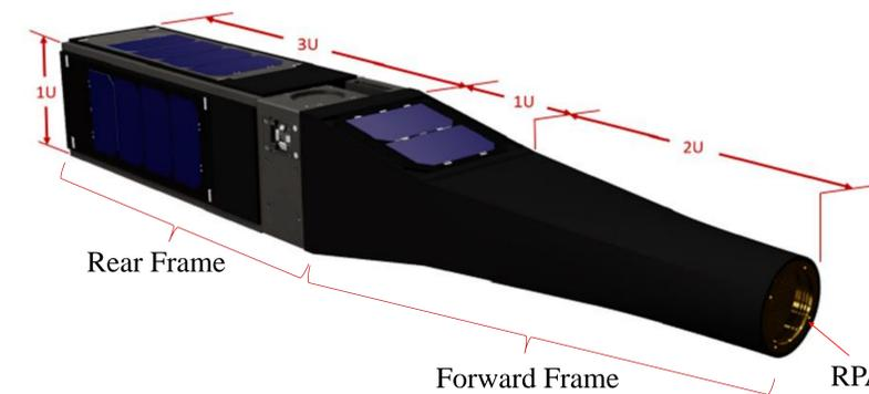
Figure 5 – The Low-Flyer is separated into a Rear Frame and Forward Frame. The Rear Frame hosts the thruster, antenna, ballast, and electronics package. The Forward Frame hosts the RPA, batteries, and GPS unit.
