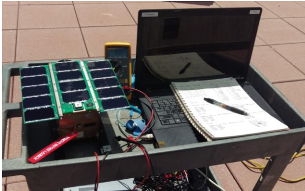
Figure 10: Challenger solar panel testing
