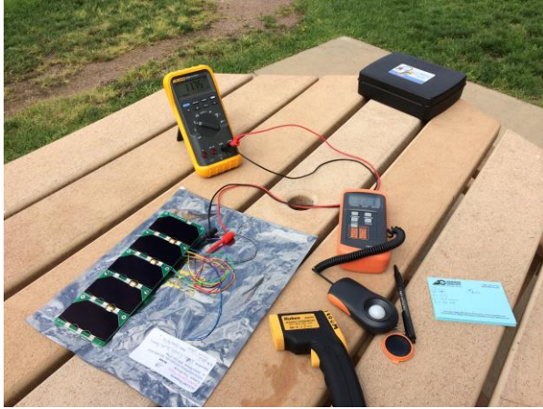
Figure 4: MinXSS solar panel testing
