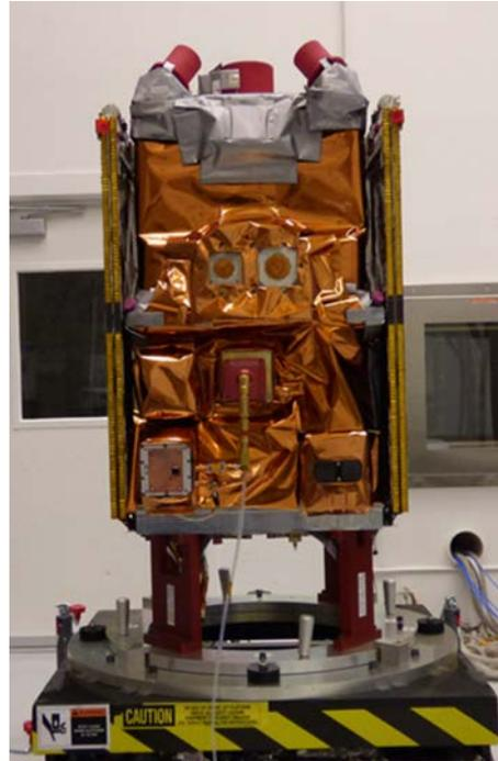
**Figure 3: GPIM Space Vehicle.** The GPIM mission leverages a flight heritage BCP-100 spacecraft and a flight demonstration AF-M315E propellant propulsion subsystem.
