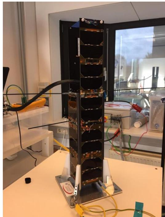
**Figure 6 : Flight model of PicSat, antennas and solar panels deployed**
