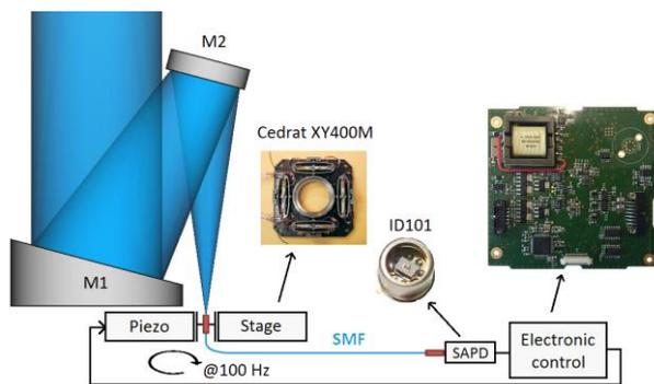
**Figure 2 : Payload control loop**
