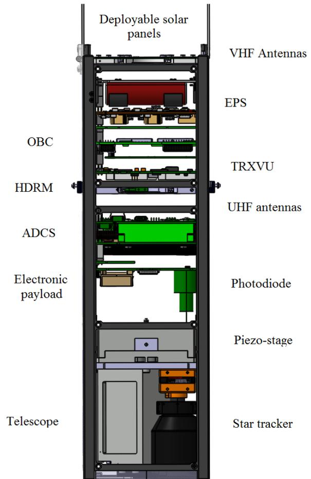
**Figure 5 : Detailed view of the full satellite**
