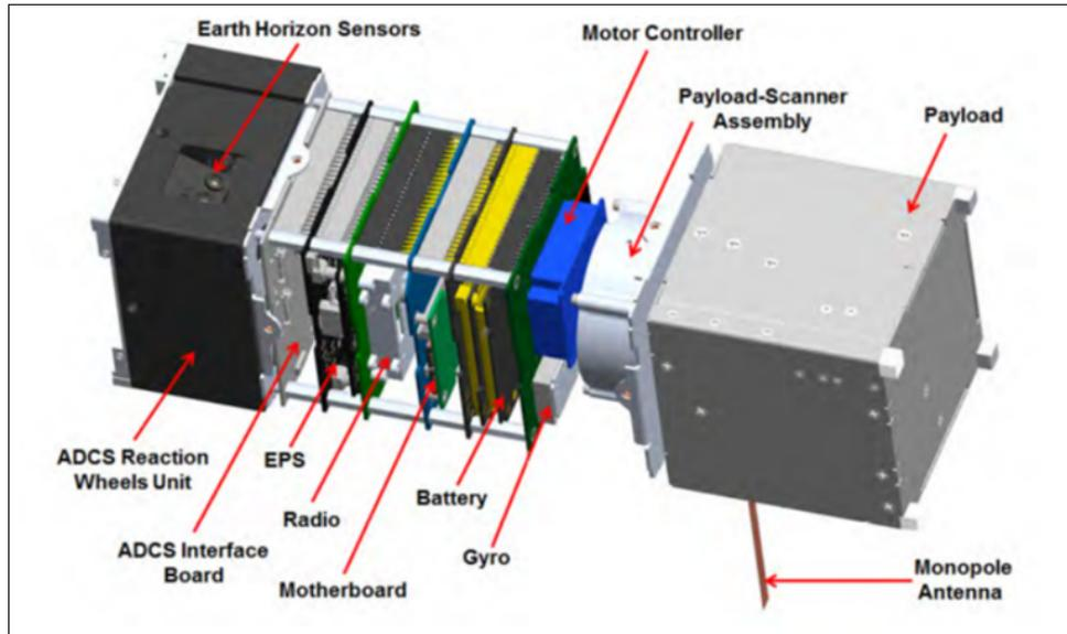
**Fig. 2.** MicroMas-2 Space Vehicle (without solar panels)
