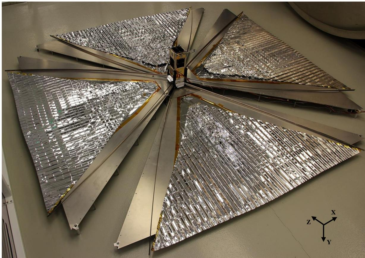
**Figure 3: CanX-7 Spacecraft with Fully Deployed Drag Sail during Testing at SFL**
