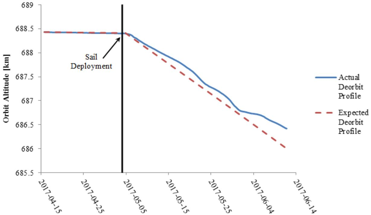
Figure 5: Preliminary Deorbit Profile for the CanX-7 Spacecraft
