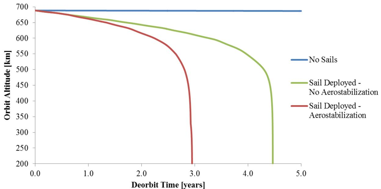
**Figure 7: Predicted Long-Term Deorbit Performance for CanX-7**
