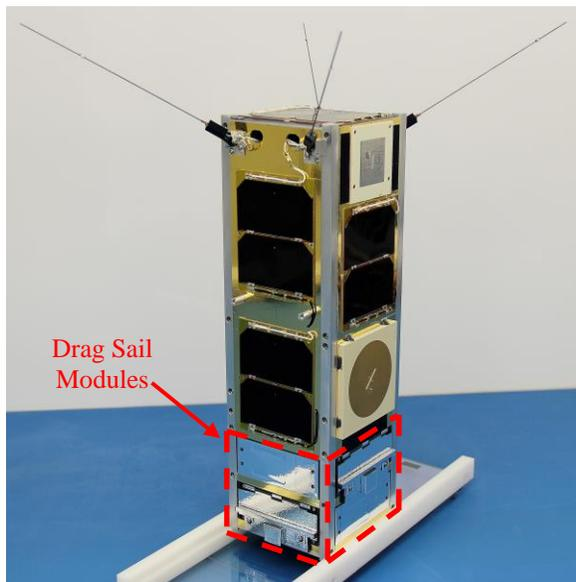
**Figure 1: CanX-7 Spacecraft in Cleanroom Prior to Launch**
