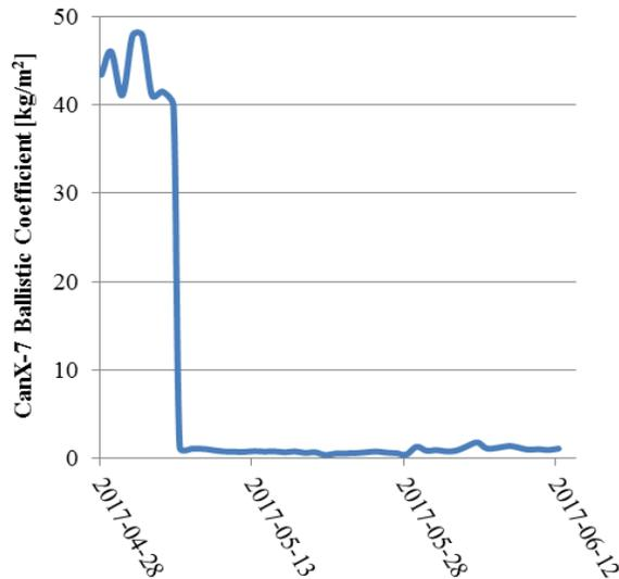
**Figure 6: Ballistic Coefficient for CanX-7 before and after Sail Deployment**
