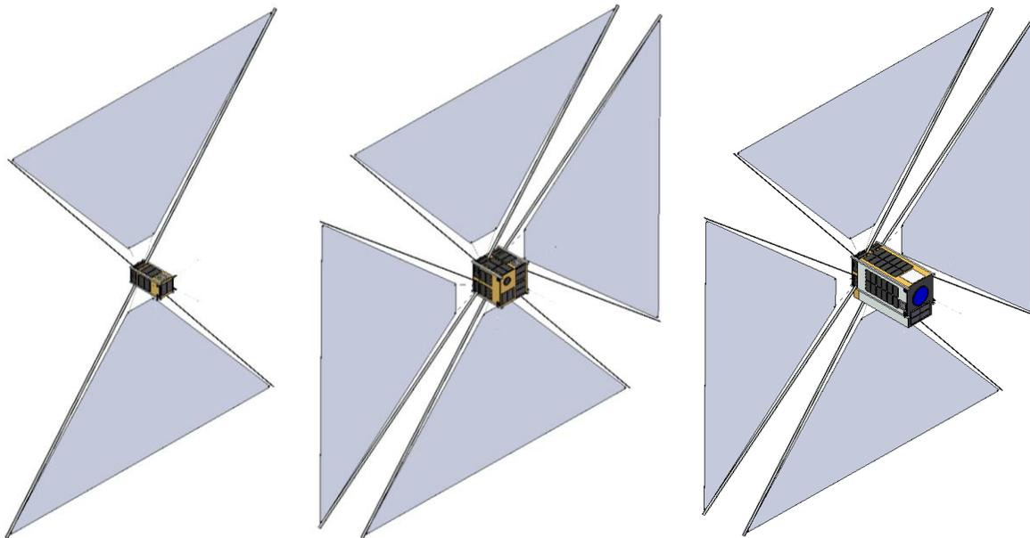
**Figure 8: Drag Sail Concepts for a Variety of Spacecraft Geometries: 2U (left), SFL GNB Class (middle), SFL NEMO class (right)**
