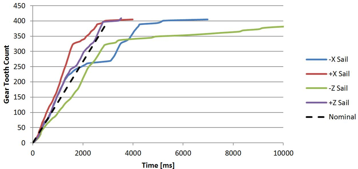
**Figure 4: On-Orbit Deployment Profiles for the CanX-7 Drag Sail Modules**
