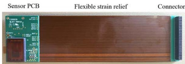
**Figure 4: Sensor Unit for the Gecko Imager**
