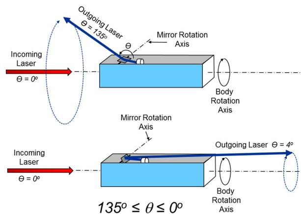
**Figure 5. Pointing geometry of an optical relay satellite using a single-axis gimbal.**
