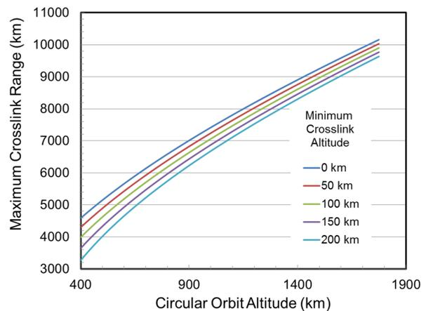
**Figure 3. Maximum possible crosslink range as a function of orbit altitude and minimum tangent height.**
