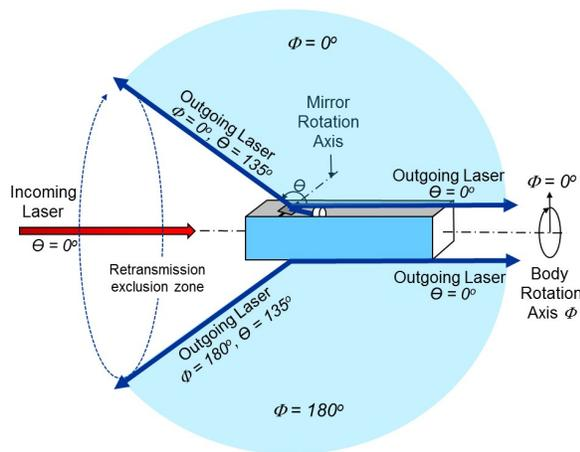
**Figure 6. Available pointing directions for the CORD satellite concept.**
