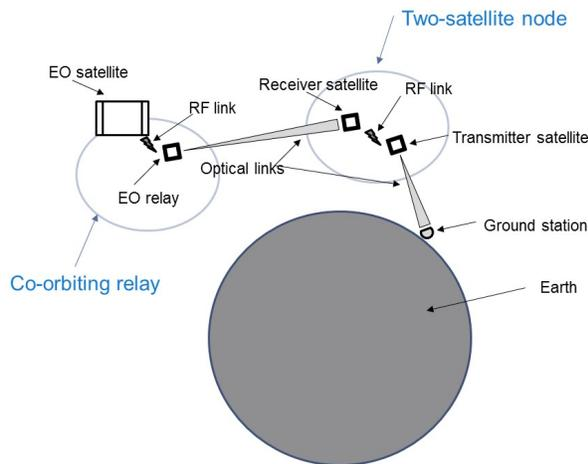
**Figure 7. Schematic representation of the use of two-satellite nodes and co-orbiting relays.**
