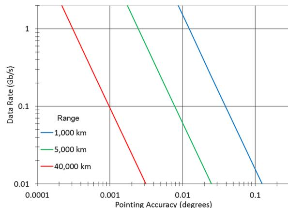
**Figure 2. Data rate capacity of an optical link from a 4-W laser to a 10-cm-diameter receiver as a function of range and transmitter pointing accuracy.**
