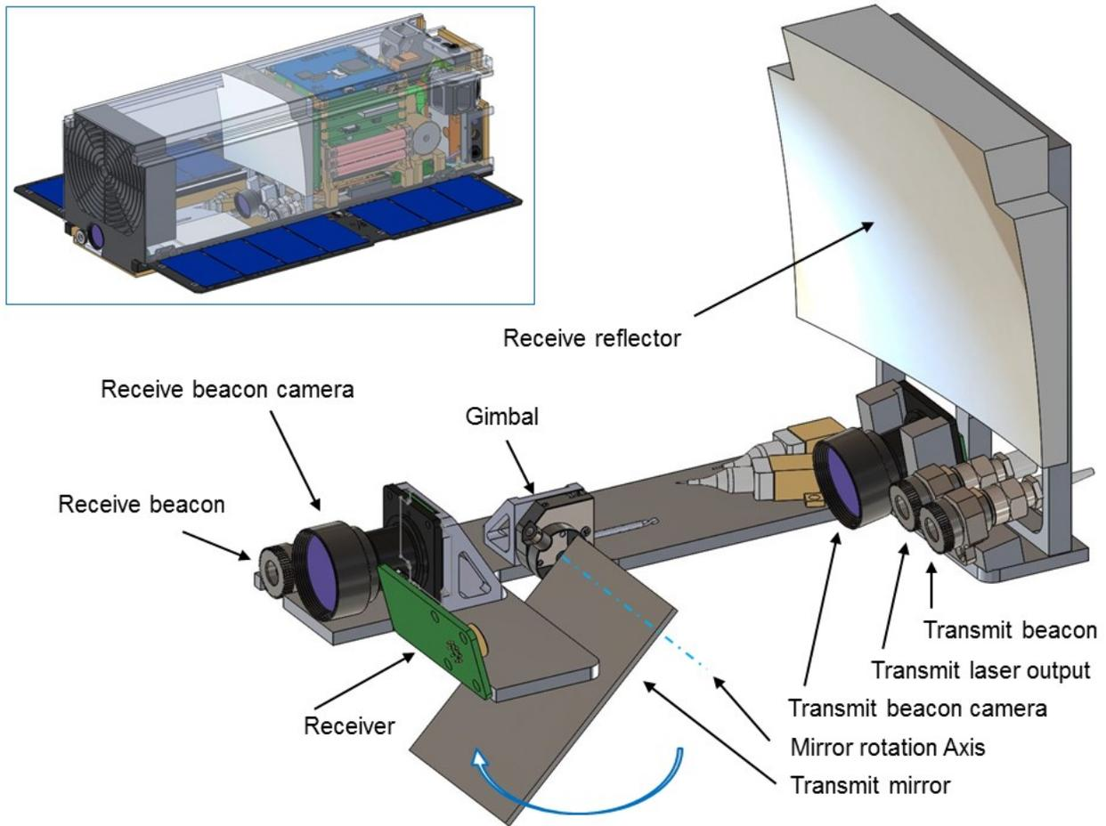
**Figure 4. Conceptual design of an optical relay satellite using a single-axis gimbal in a 3U form factor.**
