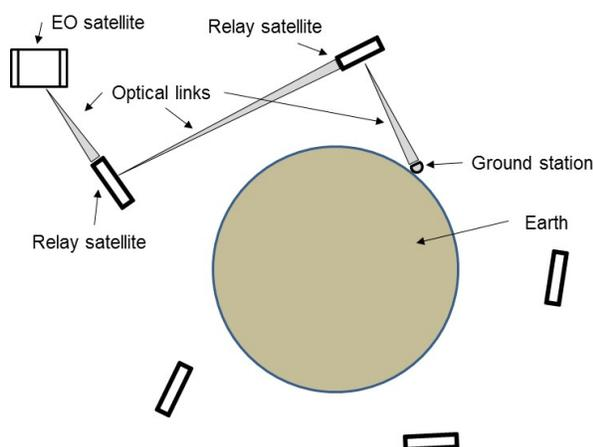
**Figure 1. Schematic illustration of a LEO optical network.**
