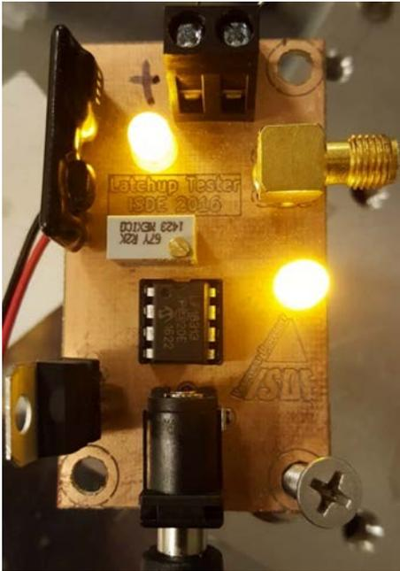
Figure 6 - Photograph of the latchup detection and correction circuit.
