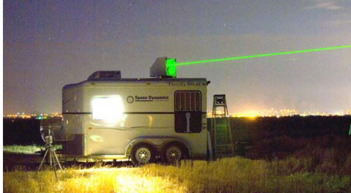
Fig. 1. The three wavelength Aglite lidar at dusk, scanning a harvested wheat field.
