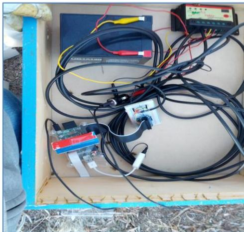
*Figure 3.1. BeePi hardware components in a Langstroth super*
