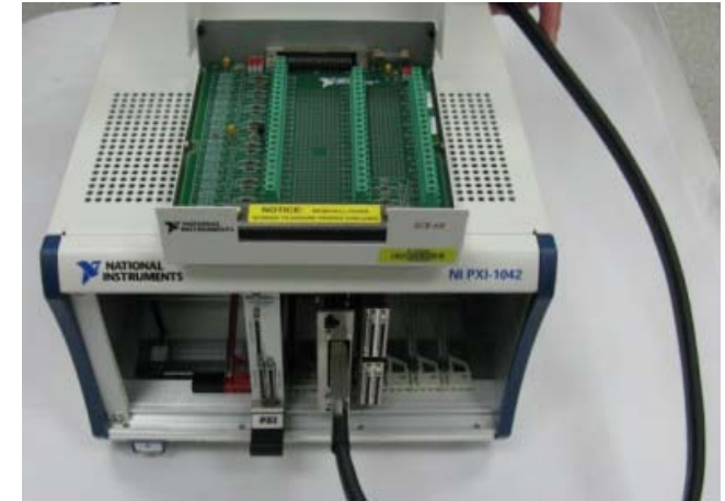
RDE & Upper Breakout installed in NI PXI-1042 chassis with NI 6868-RDIO cable and SCB-68 chassis. NI PXI-7854R board (left)
