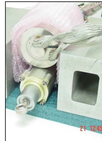
Actuator with motor, angle sensor, and LVDT
