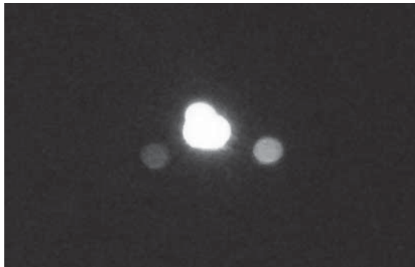
Figure 1. An aircraft on final approach (about 400 m above ground level, 3 km from runway) at night into Cleveland-Hopkins International Airport, Ohio, USA, demonstrates the position of landing lights (center) and navigation lights (red on left wing, green on right wing). (Grayscale version of cell phone photo by R. A. Dolbeer)
